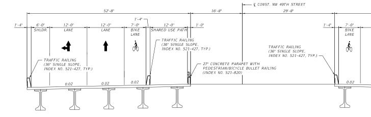
DESIGN SPEED = 45 MPH NW 49 ST STRUCTURES TYPICAL SECTION
