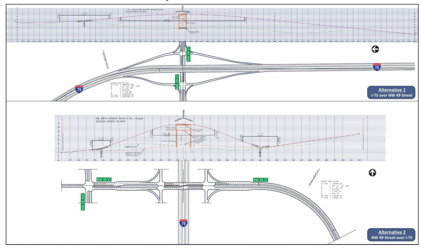
Figure 3- Alternatives 1 and 2 – Plan and Profile
