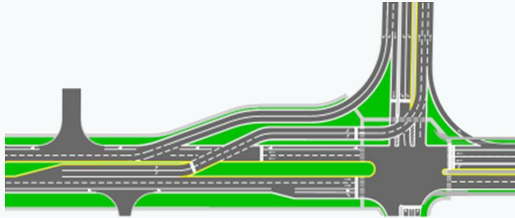
DISPLACED LEFT TURN (DLT)
